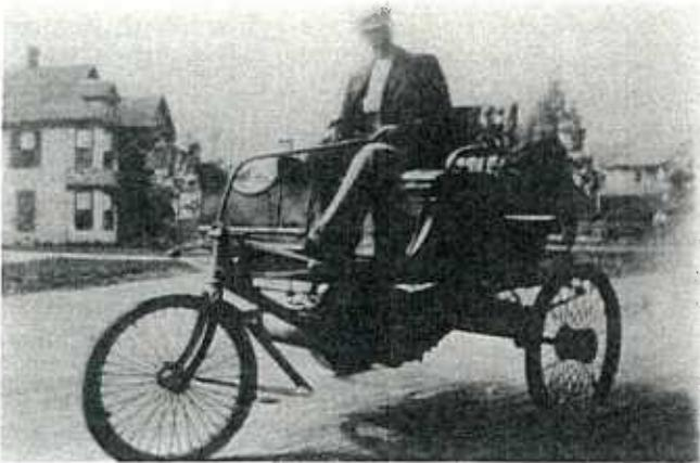
*Ray Van Auken on his 1900 Knox which was handed down through the Van Auken family. The machine ran on a 1 cylinder, air-cooled engine. On its tubeless front pneumatic tire and two 2.50 x 24 solid tires the three-wheeler could reach 8 mph when the throttle was opened wide.*
